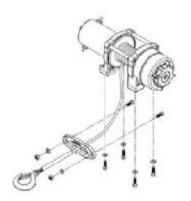
order to make sure the motor, drum and gearbox housing are aligned correctly.
