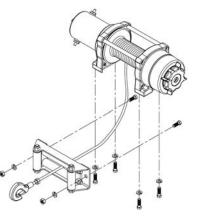
order to make sure the motor, drum and gearbox housing are aligned correctly.
